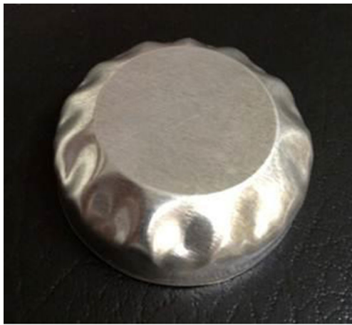
Fig. 2 Development of side-wall wrinkles in the experimental drawing of a cylindrical cup [21]
