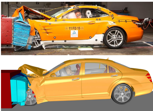
Fig. 2 Frontal impact of a car with initial speed of 64 km/h against a deformable barrier: experimental ( top ) and numerical simulation result ( bottom ) (courtesy of Daimler Chrysler AG)
